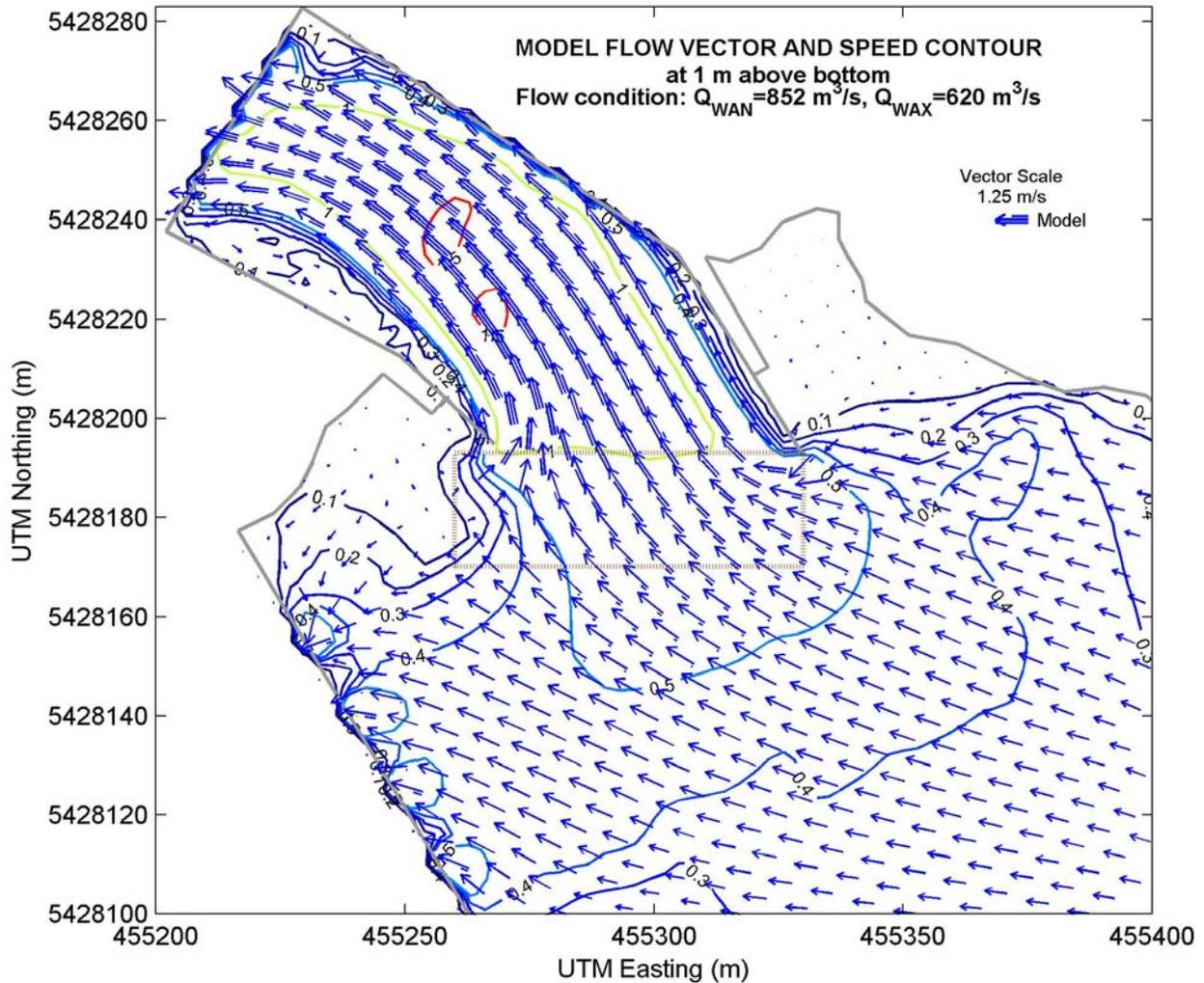
Figure 10: Model results of the headpond velocities at 1 m above bottom for a case with an existing Waneta turbine discharge of  $852 \text{ m}^3/\text{s}$  and a WEP turbine discharge of  $620 \text{ m}^3/\text{s}$ .
