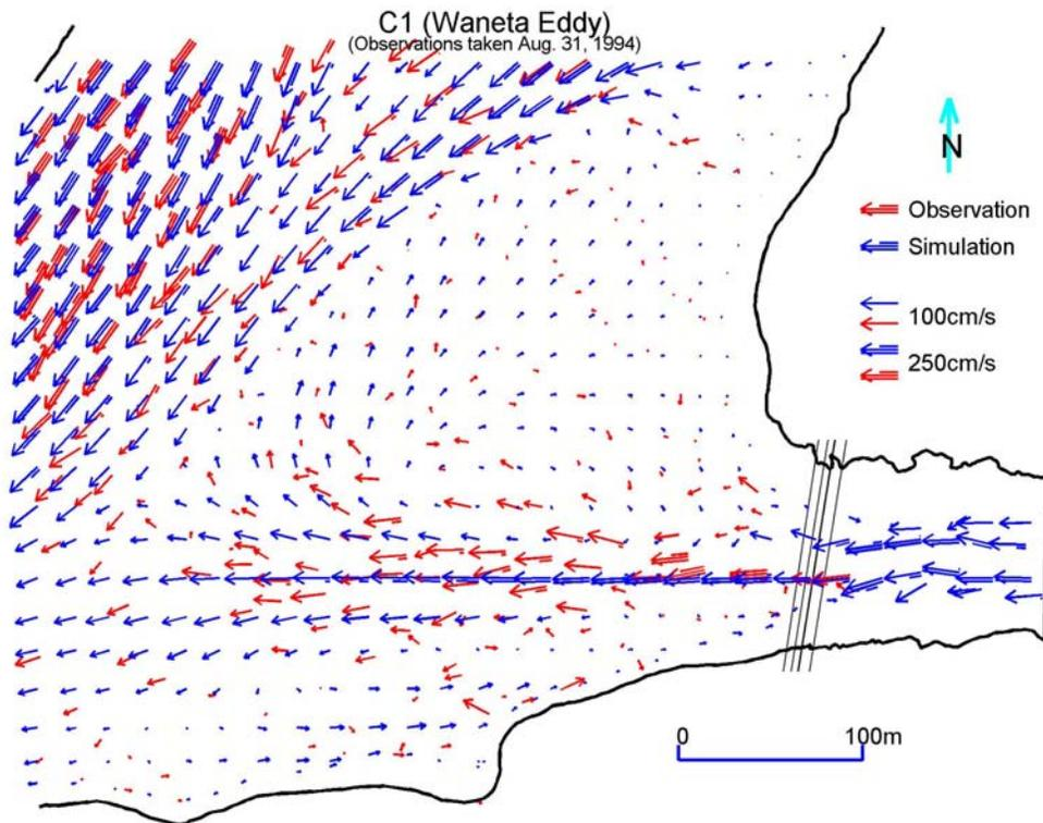
Close-up of the Waneta Eddy with Simulated flows at a depth of 2.2 m
