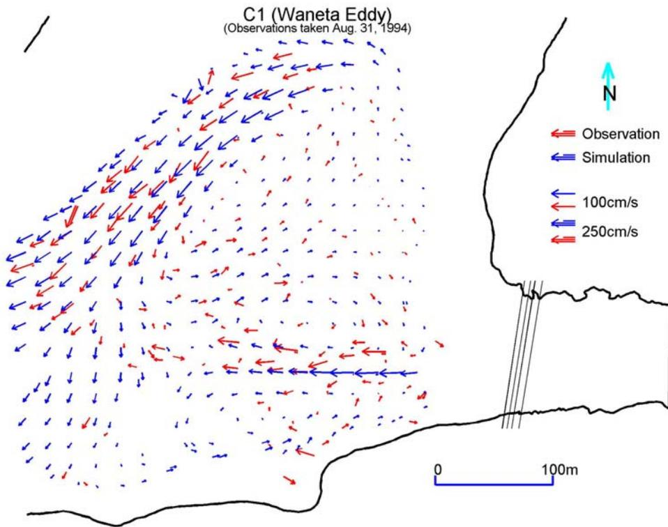
Close-up of the Waneta Eddy with Simulated flows at a depth of 8.2 m
