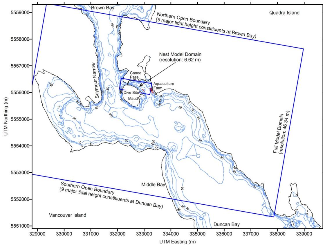
**Figure 4:** The model domain used for the Canoe Pass sediment simulations. Canoe Pass separates Maud Island from Quadra Island in the Discovery Passage area east of Vancouver Island B.C.
