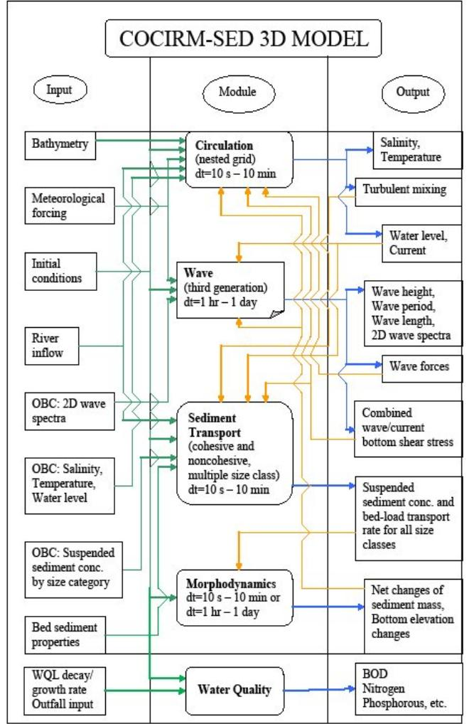
**Figure 1: Schematic diagram of the COCIRM-SED numerical model.**
