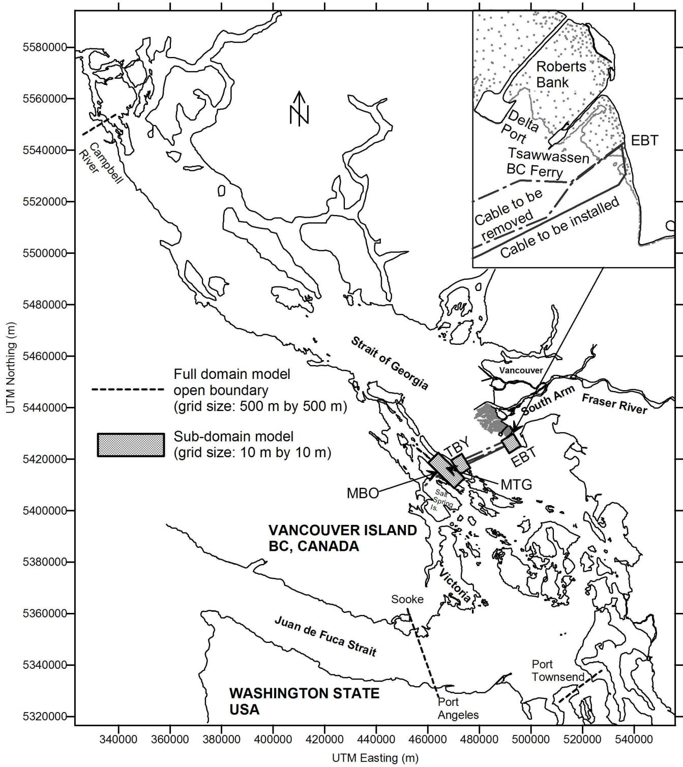
**Figure 2: A map of the study area showing the existing underwater transmission cables and the COCIRM-SED basin scale model domain and the high resolution sub-domains at EBT, TBY and MBO landing sites.**
