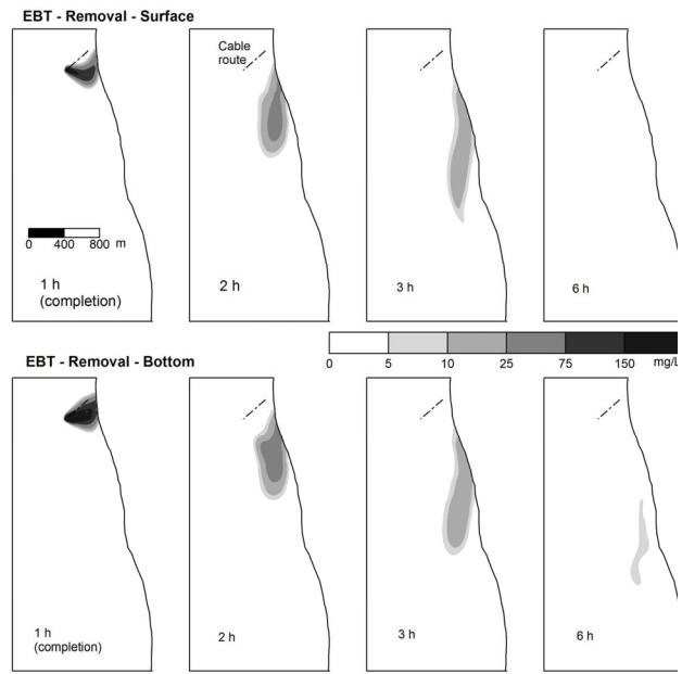
**Figure 3: Sediment plumes associated with cable removal at EBT.**
