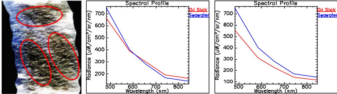
**Figure 5.** Response of sub-surface oil slicks or light oil surface traces. (Left) CASI image; (Middle) “Spectral rotation”; (Right) Spectral “rotation” + absorption.
