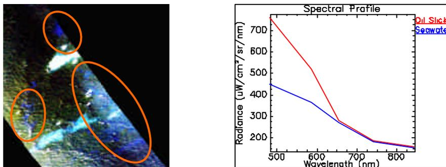
**Figure 4.** Response of a surface oil slick. (Left) CASI image; (Right) Spectral signature illustrating the fluorescence in the blue.
