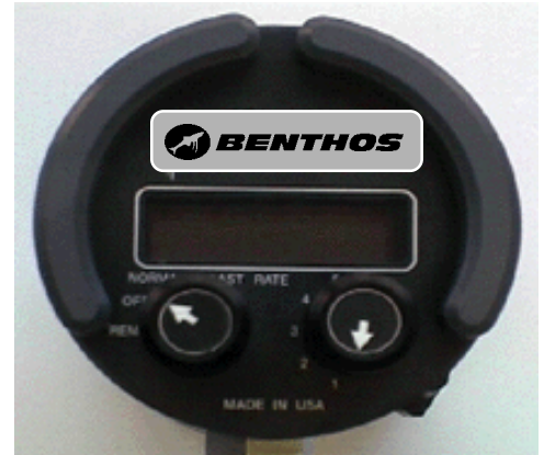
LCD displays range in meters, directional bearing, transmit and receive functions, channel selection, and low battery indicator.
