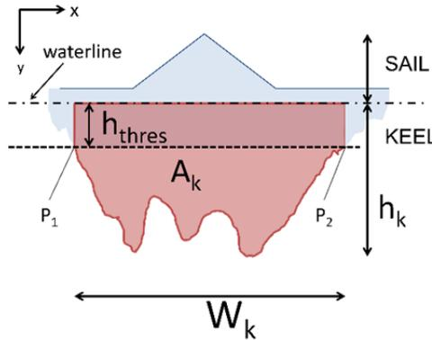
**Figure 2: The schematics of the ridge keel geometry where  $h_k$  is the ridge keel draft,  $w_k$  the keel width and  $A_k$  the keel area (After Ekeberg et al., submitted).**
