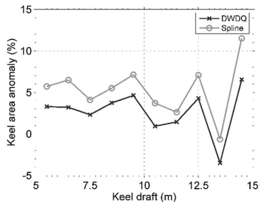
Figure 7: Anomalous keel area vs. draft compared with the running average (minimum 5 ridges per bin, 1 m bin size)
