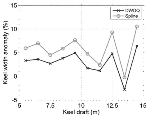
Figure 6: Anomalous keel width vs. draft compared with the running average method (minimum 5 ridges per bin, 1 m bin size).
