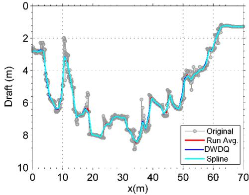
Figure 3: High resolution results, the drift speed was 0.02 m/s while the measurement frequency was 1/3 Hz.
