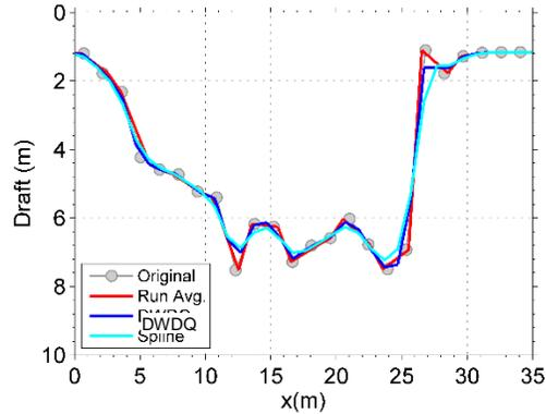
Figure 4: Low spatial resolution results, the drift speed was 0.41 m/s while the measurement frequency was 1/3 Hz.
