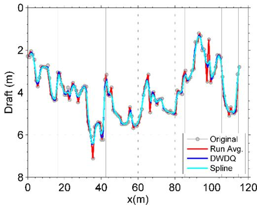
Figure 5: The 5 minute section measured 06:45 21st November 2010. The grey lines in the background indicate the start/end of an ice ridge analysing the data which were smoothed with the running average.
