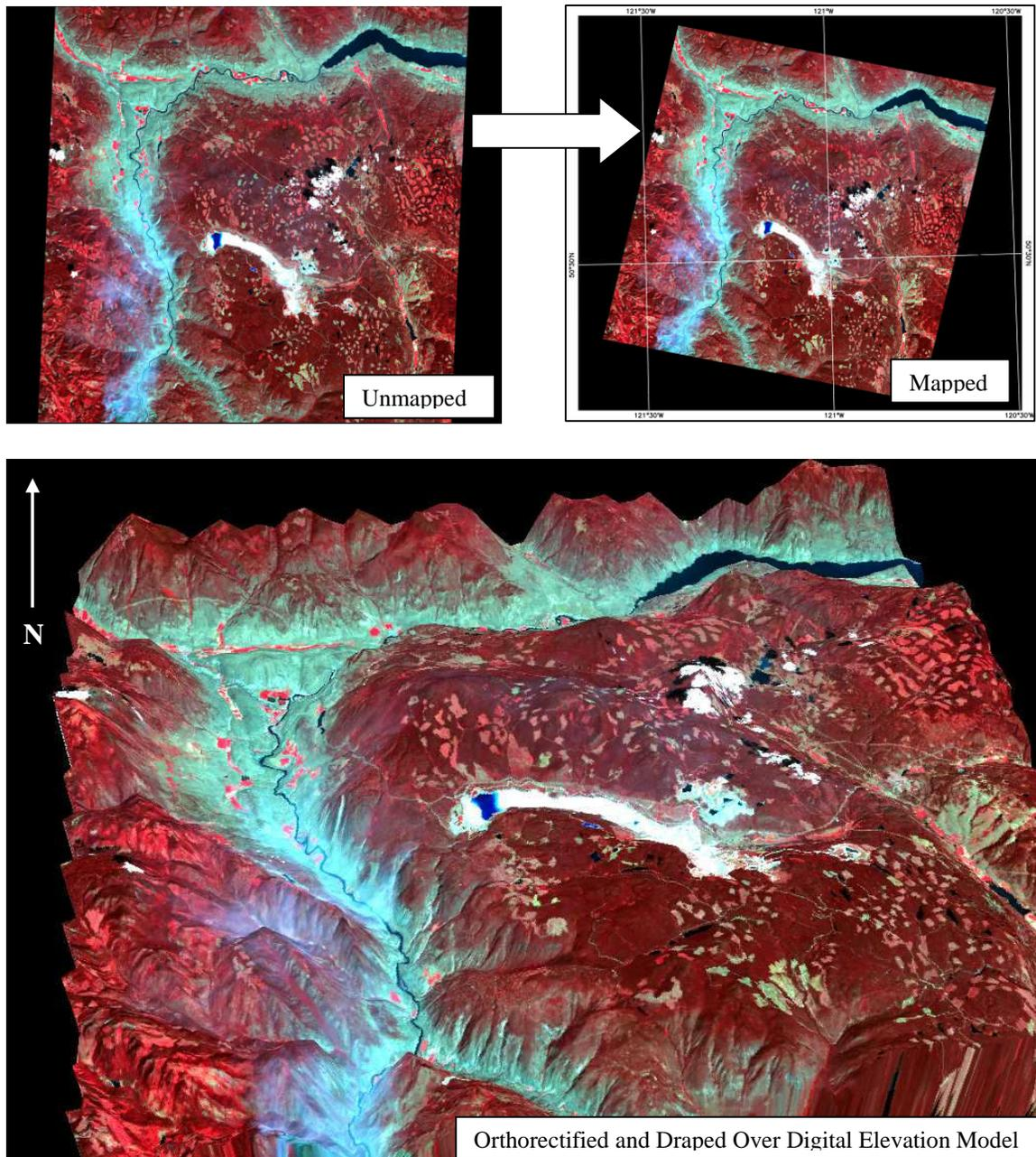
**Figure 2.** Example of mapping and orthorectification of ASTER Colour Infrared (CIR) image draped over a digital terrain model.
