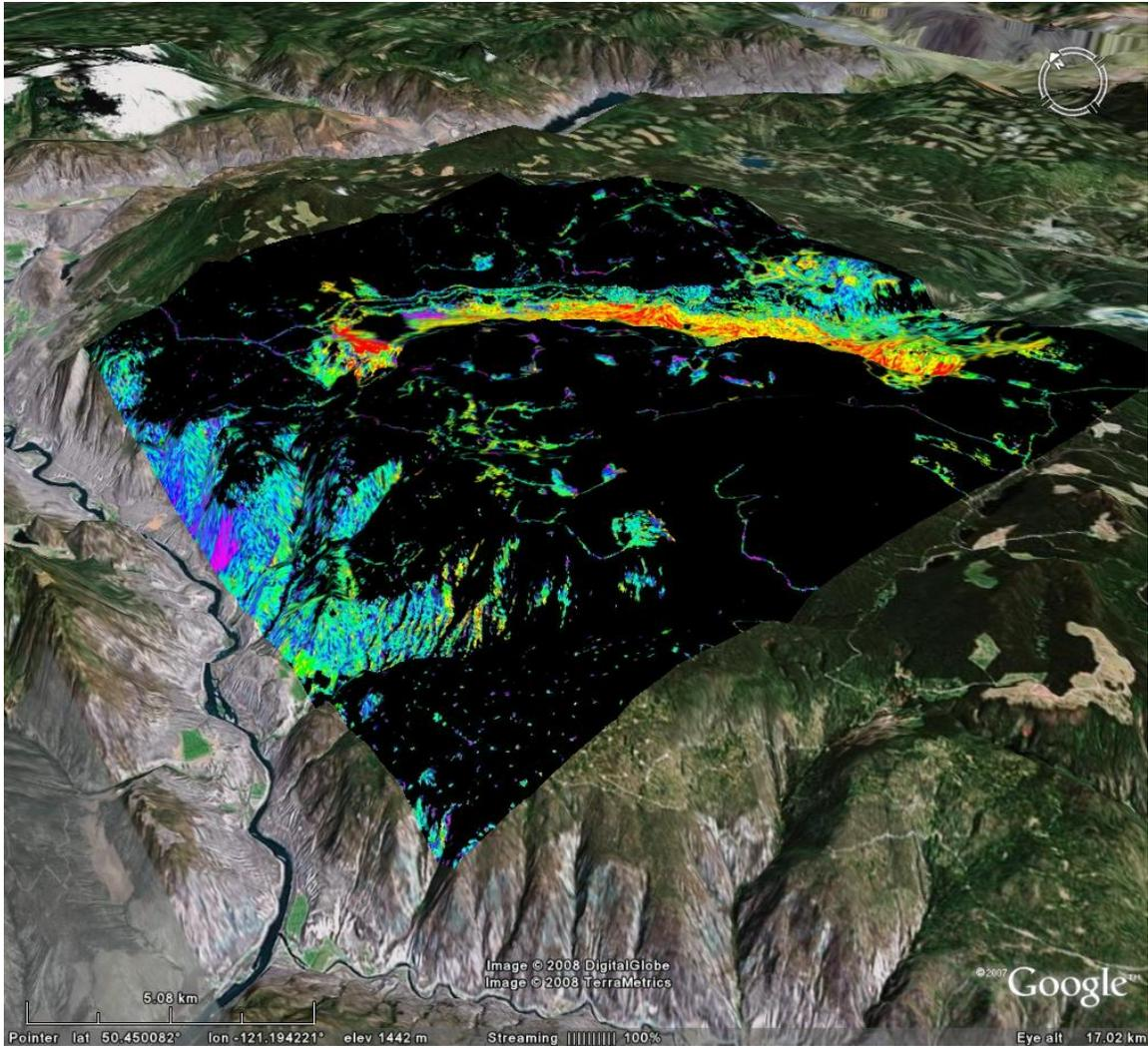
**Figure 5.** Example of the Kaolinite alteration product overlaid on a Digital Elevation Modal in Google Earth - shown as a 3-Dimensional view.
