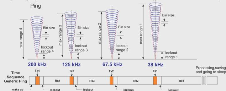
Fig. 2: Operation of 4-channel sequentially pinging sonar system. Ping rates, bin sizes, and maximum range are all programmable. Data are stored internally for easy upload to a computer following a given study.
