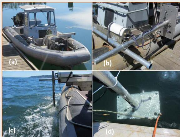
Fig. 1: (a) 23' RHIB equipped with oceanographic sampling gear. (b) Strut out of water showing AZFP electronics housing and mounting plate with acoustic transducers. (c) Strut in water and moving at 2m/s. (d) Bottom of mounting strut with transducers seen from above.
